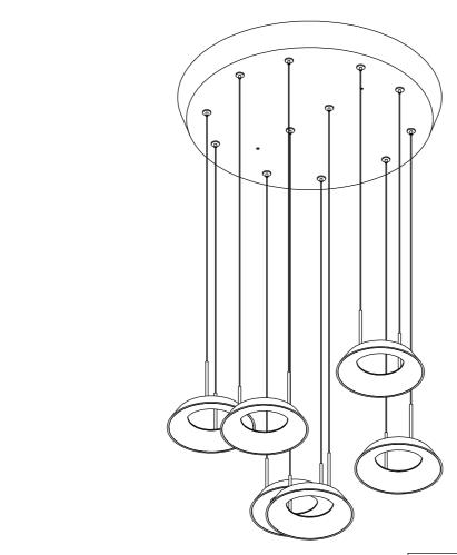
WARNING: WIRES NEED TO BE CONNECTED TO DRIVER FOUND IN CANOPY AND SHOULD NOT CONNECT DERECTLY TO POWER SOURCE OR A SHORT MIGHT OCCUR.
