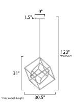
: 30.5" L x 30.5" W x 31" H : 120" OAH CANOPY : 9" W x 1.5" H x 9" L HANGING WEIGHT : 8.36 lb LAMPING INPUT VOLTAGE : 120V : 3,990 Rated (2,850 Del.) : 1 x 57W LED PCB Integrated , 57W Total BULB INCLUDED : (Integrated) DIMMABLE : Triac CL : 80+ CRI COLOR\_TEMP : 3000K
