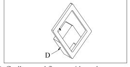
Step.4: Caulk around fixture with outdoor silicone sealant to prevent water intrusion. Leave a small gap at the bottom to allow moisture to escape. Install fixture to back plate (B) and tighten mounting screws (D) to secure.
